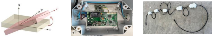
Fig. 3 Clinometer working principle [8] (left), MEMS detail (center) and sensors used in the tests (right)
