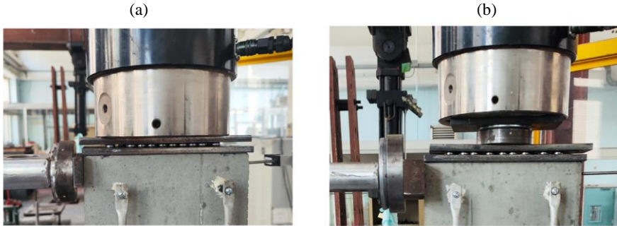
Fig. 4 Application of axial load: (a) roller support device loaded by the hydraulic jack; (b) axial spherical plain bearing coupled with roller support device.
