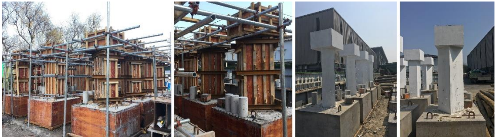
Fig. 4 Preparation of the specimens for biaxial tests.
