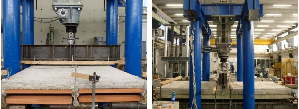
Fig. 2 Setup used for floor bending tests.
