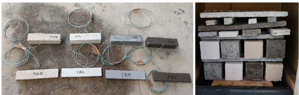
Fig. 3 Mortar prisms and TRM coupons with K-type thermocouples (left). Arrangement of specimens within the furnace (right).
