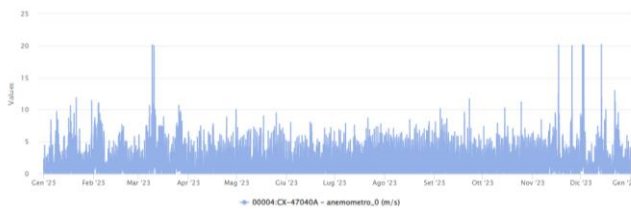
Fig. 8 Wind velocity time history over a time span of one year. Unit: [m/s]
