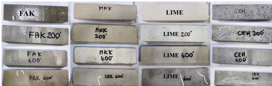
Fig. 5 Mortar prisms after exposure to high temperatures (cracks highlighted in white).
