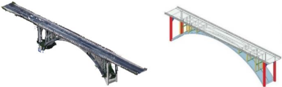
Fig. 3 BIM model superimposed by point cloud (left) WBS classification on BIM model (right)
