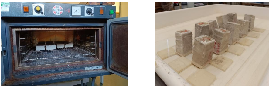
Fig. 2 Capillary absorption test: (left) specimens dried in the oven and (right) immersed in the water.
