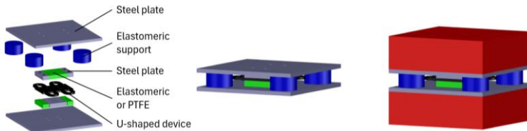
Fig. 6 U-shaped device for column-to-column connection. The system consists of two external steel plates and elastomeric supports coupled with the device. The device is anchored to the upper column through its external flanges and to the bottom column via the central plate.
