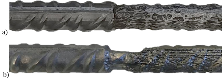
Fig.6 Corrosion morphology: a) uniform “BN2”, b) localised “C3”.
