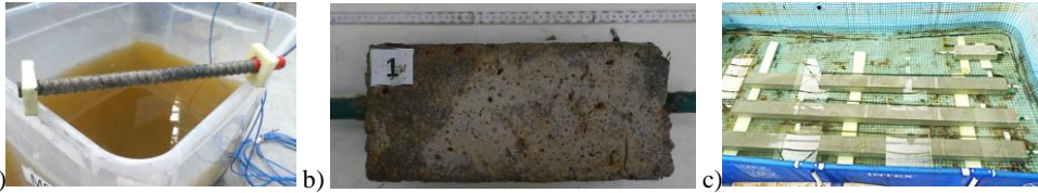
Fig.1 Specimens: a) bare bar, b) prismatic element, c) tie beam element.
