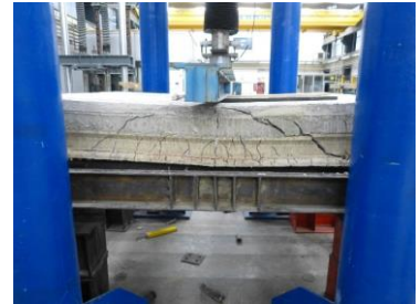
Fig. 6 Residual displacement (left) and post test condition of the F2 floor.
