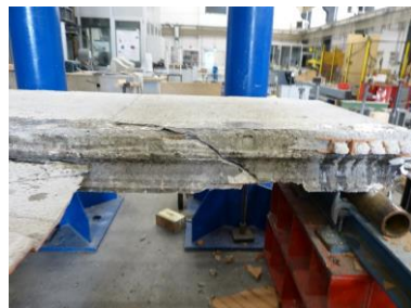
Fig. 4 Residual displacement (left) and evidence of slab shear failure mechanism (right) for the F1 floor.
