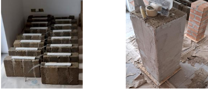
Fig. 3 Preparation of the specimens for the (left) bond and (right) compression tests.
