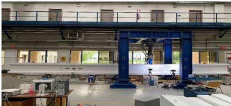
Figure 2 - Third-point bending test of a PC beam.
