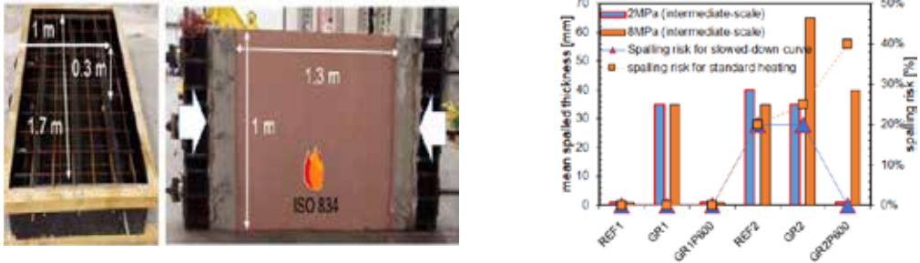
Figure 3. (left) Intermediate-scale spalling test, and (right) cross-comparison between two different scales.
